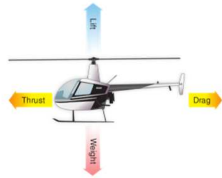
Four Main Aerodynamic Forces Acting on All Helicopters
