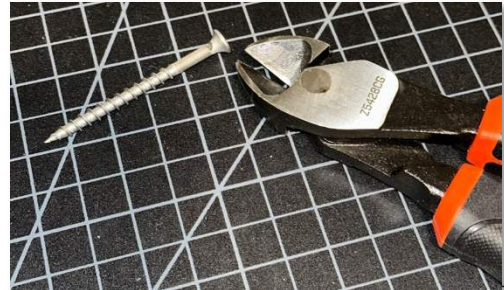
Here's a screw with the head ready to be cut off. A good pin substitute.
