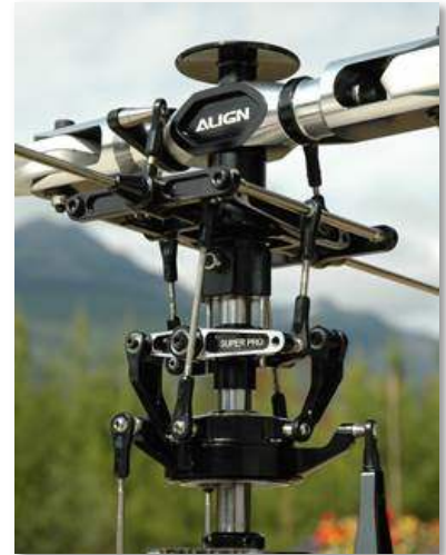
The Swashplate & Rotor Head Provide Collective & Cyclic RC Helicopter Control
